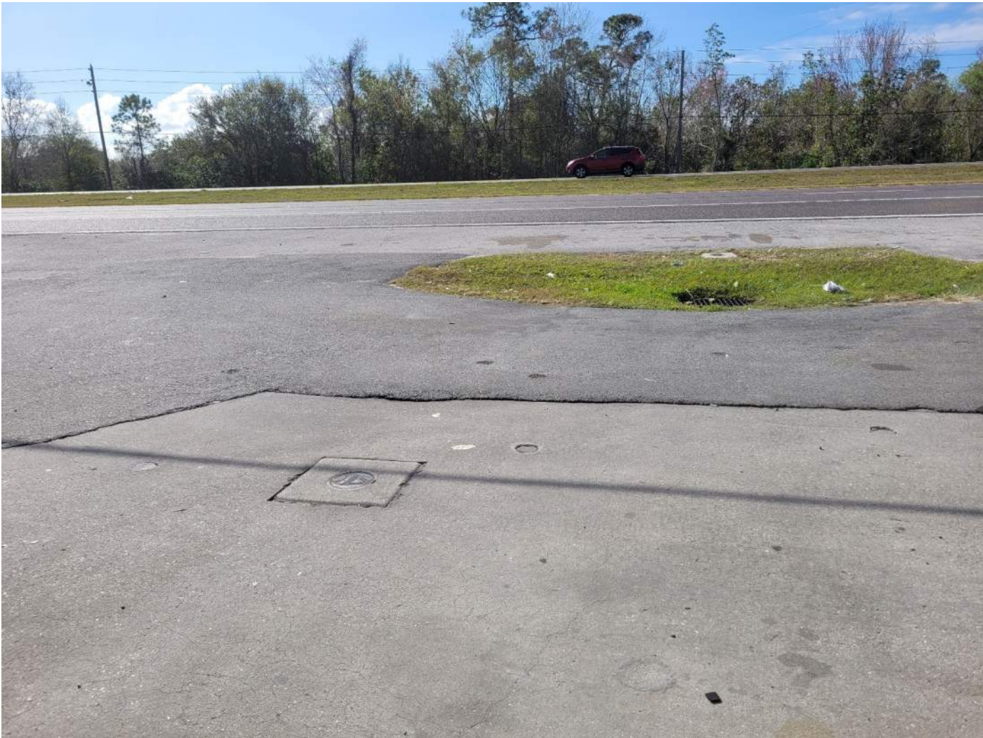
Map ID 21: Multiple monitoring wells located throughout the site
