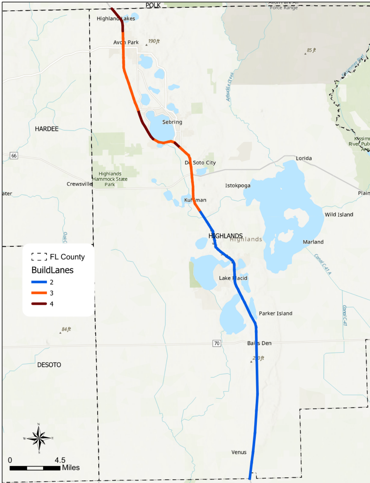
Figure 22: Build Alternative Lanes (Each Direction)
