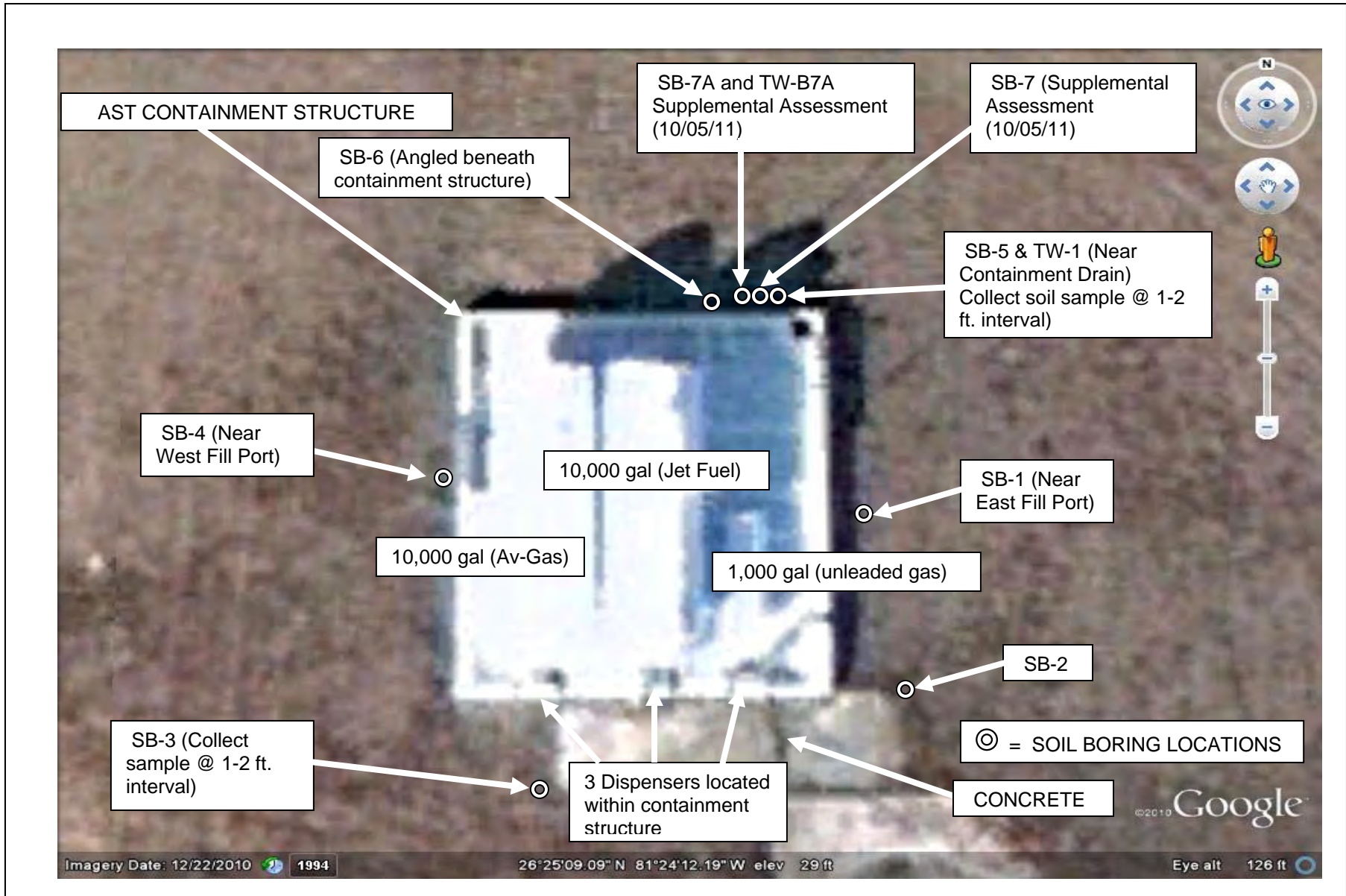
FIGURE 1. BORING LOCATION MAP BREITBURN /AIRWORKS-IMMOKALEE AIRPORT-AST CLOSURE ASSESSMENT 165 AIRPARK BLVD. IMMOKALEE, COLLIER COUNTY, FL Source: Google Earth Image - 2011; ECT, 2011
