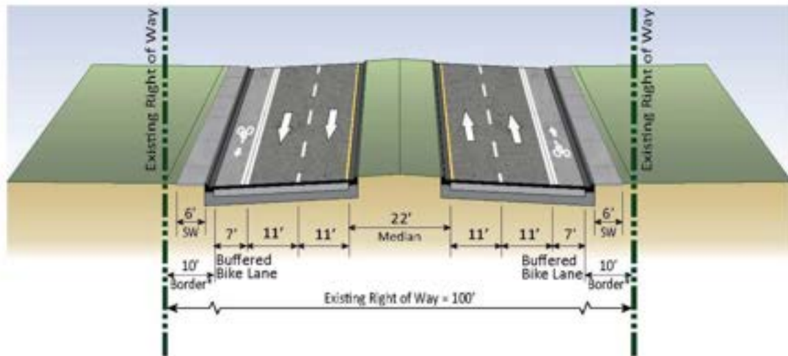
Figure 6.3 SR 29 Typical Section from North of Seminole Crossing Trail to South of CR 846
