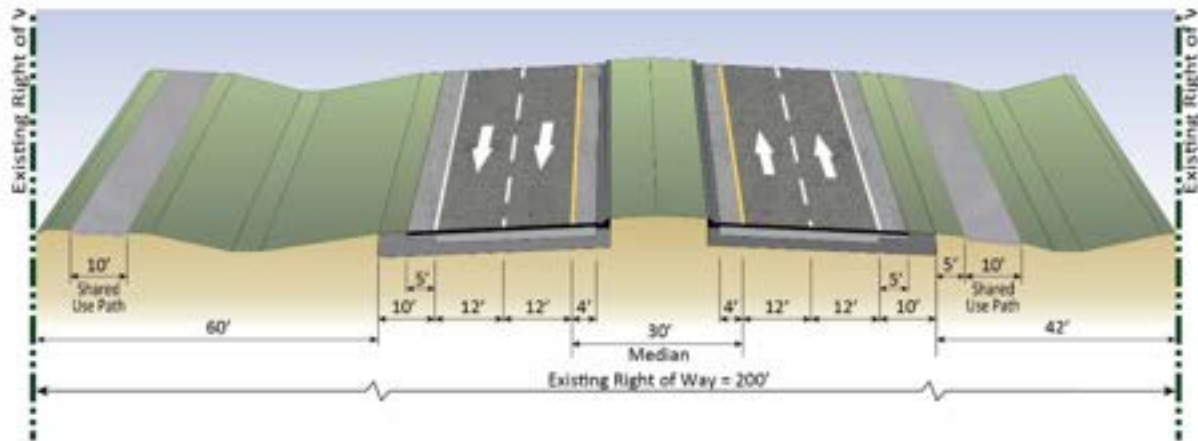
Figure 6.4 SR 29 Typical Section from South of Westclox Street/New Market Road W to Heritage Boulevard
