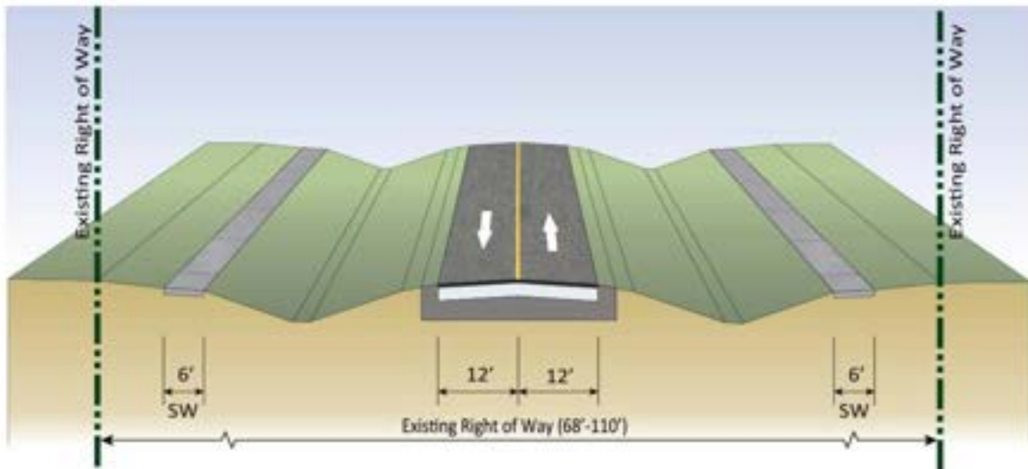
Figure 2.7 New Market Road Existing Typical Section from SR 29 South to SR 29 North
