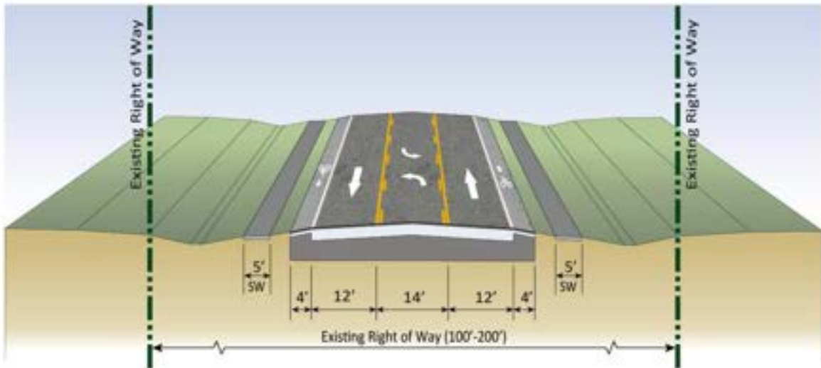
Figure 2.5 SR 29 Existing Typical Section from North 9 th Street to Westclox Street/New Market Road W
