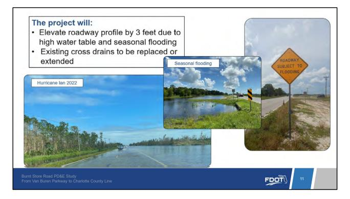
The roadway profile will be elevated approximately three feet to account for the high water table in the area and a history of flooding events. The existing nine cross drains, which include the bridge culvert over Yucca Pens Creek, will be extended or replaced. The culvert elevations and sizes will be appropriately designed to maintain the east to west hydrological flows of the area. A stormwater management system with stormwater ponds and floodplain compensation sites will be provided.
