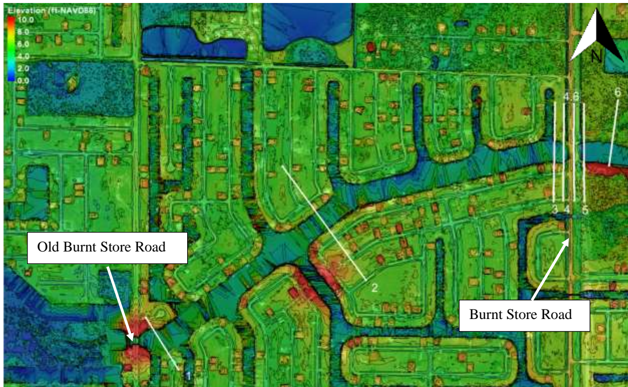
Figure 2-4 LiDAR Elevation Contours and HEC-RAS Model Cross-Sections (White)
