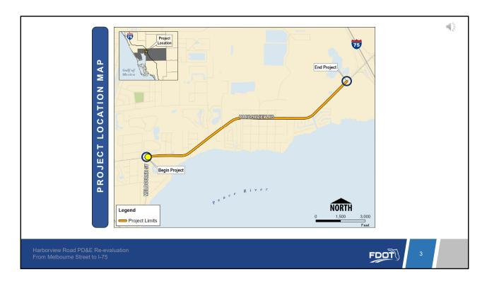
FDOT is preparing final design plans for Harborview Road from Melbourne Street and extending 2.3 miles to I-75, in Charlotte County. FDOT proposes to widen Harborview Road from the existing two-lane, undivided roadway to a four-lane, divided roadway with the addition of roundabouts at Melbourne Street and Frontage Road. Both Harborview Road and Melbourne Street are under the jurisdiction of Charlotte County.
