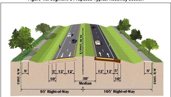
Figure 4.6: Segment C Proposed Typical Roadway Section
