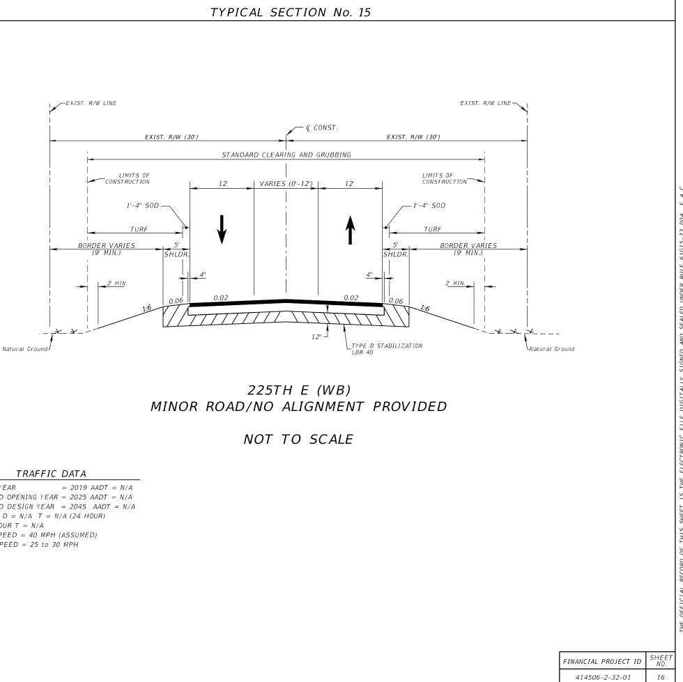
CURRENT YEAR ESTIMATED OPENING YEAR = 2025 AADT = N/A ESTIMATED DESIGN YEAR = 2045 AADT = N/A K = 9.5% D = N/A T = N/A (24 HOUR) DESIGN HOUR T = N/ADESIGN SPEED = 40 MPH (ASSUMED)POSTED SPEED = 25 to 30 MPH
