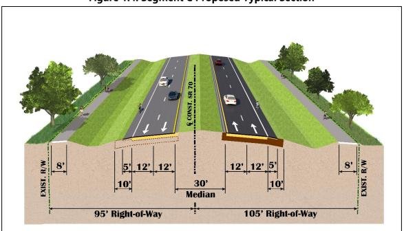
Figure 1.4: Segment C Proposed Typical Section
