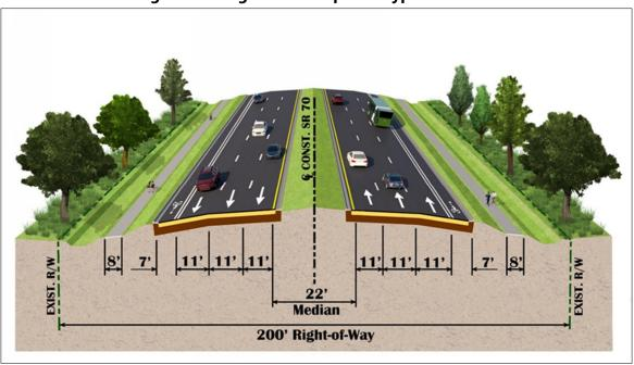
Figure 1.2: Segment A Proposed Typical Section
