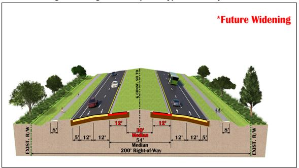
Figure 4.5: Segment B Proposed Typical Roadway Section
