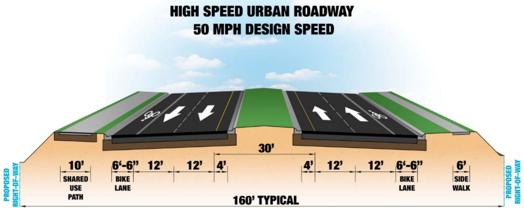
Figure 6. Design Typical Section – SR 710 from E. of Taylor Creek to the L-63N Interceptor Canal
