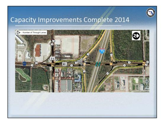
This illustration shows the improvements currently under construction. The "no-build" alternative assumes that aside from ongoing widening scheduled for completion in 2014, no additional improvements are made to the I-75 and State Road 951 interchange through the year 2035 ("twenty thirty-five").
