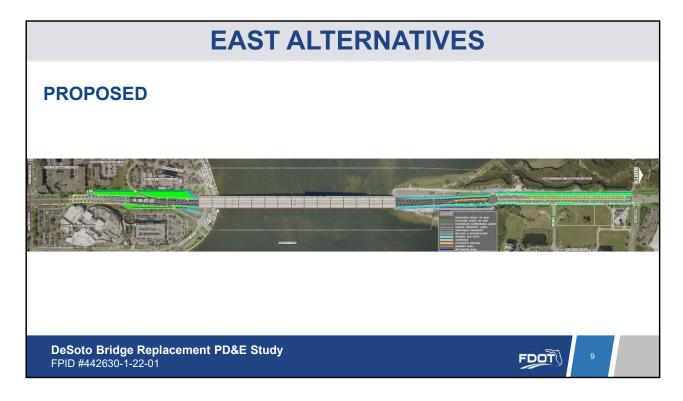
The east alternative includes constructing the first phase of the replacement bridge to the east of the existing bridge and slightly east of the current roadway connection. Approximately 0.6 acres of total right of way is needed along the roadway on the south and north side of the river.
