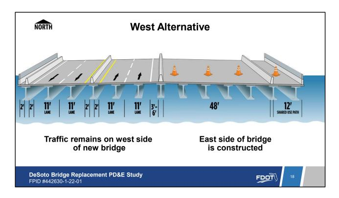
Once the old bridge is removed, the second half of the new bridge will be constructed and joined with the new bridge built in Phase 1 to complete the new structure.
