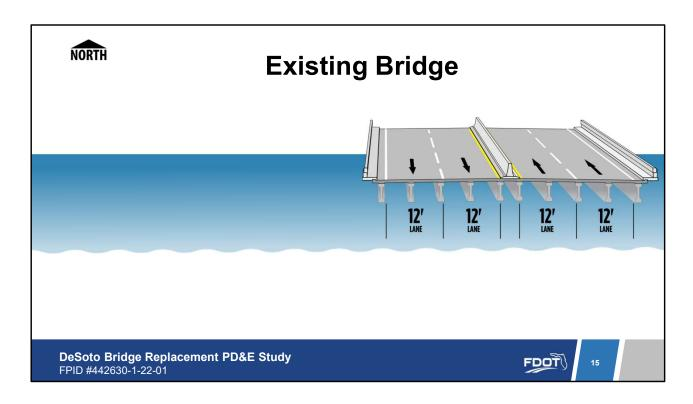
The existing bridge has two travel lanes in each direction. The new bridge will be built on either the WEST or EAST side of the existing bridge.
