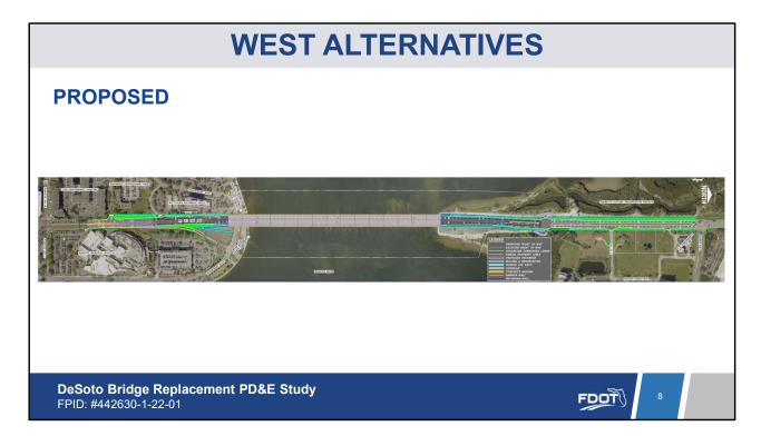
The west alternative includes constructing the first phase of the replacement bridge to the west of the existing bridge and slightly west of the current roadway connection. Approximately 0.4 acres of total right of way is needed along the roadway on the south and north side of the river.
