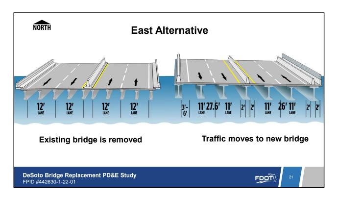
Once this is complete, traffic will be switched to the new bridge which will accommodate two travel lanes each direction and a shared use path but will not have shoulders. After traffic is shifted onto the new bridge, the demolition of the old bridge will occur.
