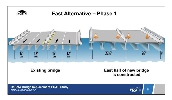
The first phase of construction for the EAST alternative includes building half of the bridge and one side of the shared use path to the east of the existing bridge.
