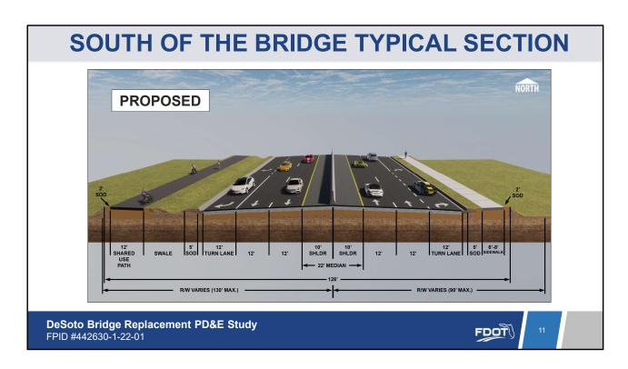
South of the Bridge the typical section includes two 12-foot travel lanes and two 12-foot turn lanes in each direction, a shared use path on the east side of the road and a 6-to-8-foot sidewalk on the west side of the roadway. The typical section also includes 10-foot inside shoulders and a swale on the west side of the road for drainage.
