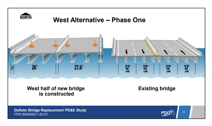
The first phase of construction for the west alternative includes building half of the bridge and one side of the shared use path to the WEST of the existing bridge.
