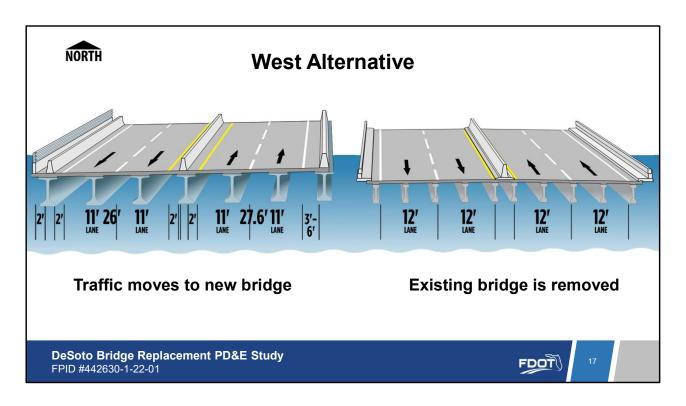
Once this is complete, traffic will be switched to the new bridge which will accommodate two travel lanes each direction and a shared use path but will not have shoulders. After traffic is shifted onto the new bridge, the demolition of the old bridge will occur.
