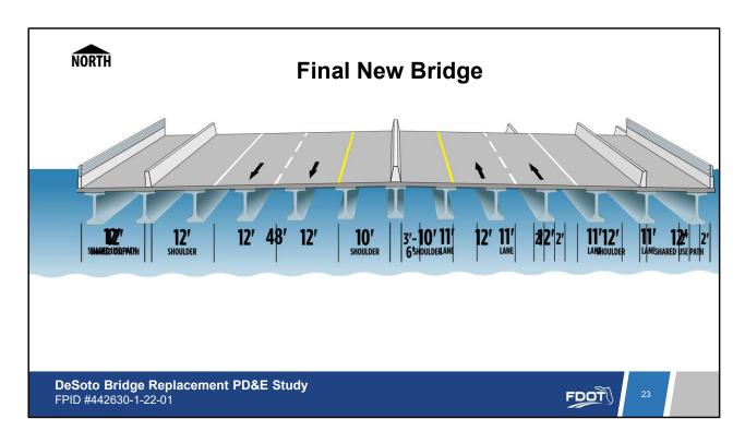
New striping will be placed on the entire bridge structure and traffic will be switched to the new bridge.
