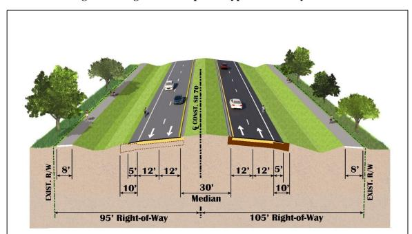
Figure 4.3 Segment C Proposed Typical Roadway Section
