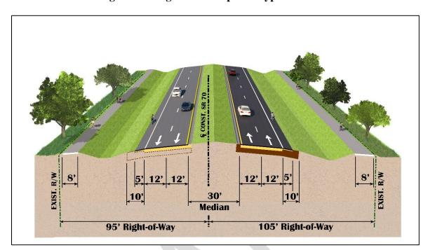
Figure 1.4: Segment C Proposed Typical Section
