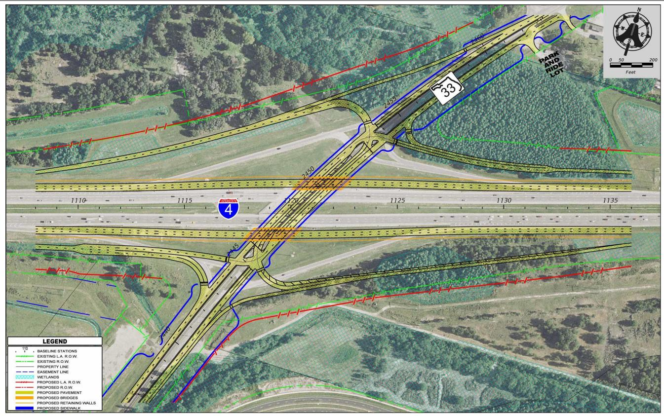
FIGURE 7-3: BUILD ALTERNATIVE NO. 1 (DIAMOND INTERCHANGE)
