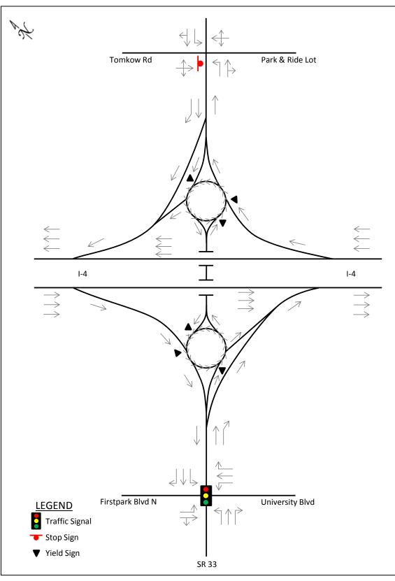
FIGURE 7-2: DESIGN YEAR (2036) INTERCHANGE/INTERSECTION GEOMETRY – TSM ALTERNATIVE
