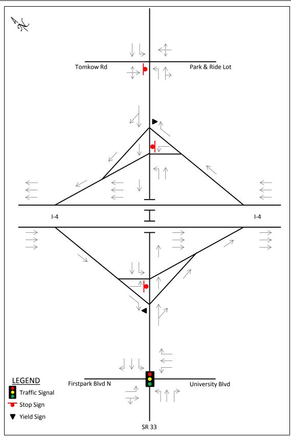
FIGURE 2-2: EXISTING YEAR (2012) INTERCHANGE/INTERSECTION GEOMETRY
