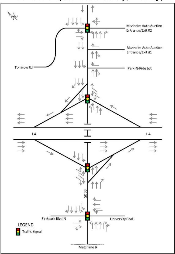
Figure 5-15 Build Alternative Proposed Intersection Geometry (I-4 Interchange)
