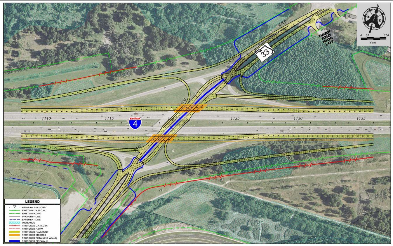
FIGURE 7-10: BUILD ALTERNATIVE NO. 2 (DIVERGING DIAMOND INTERCHANGE)
