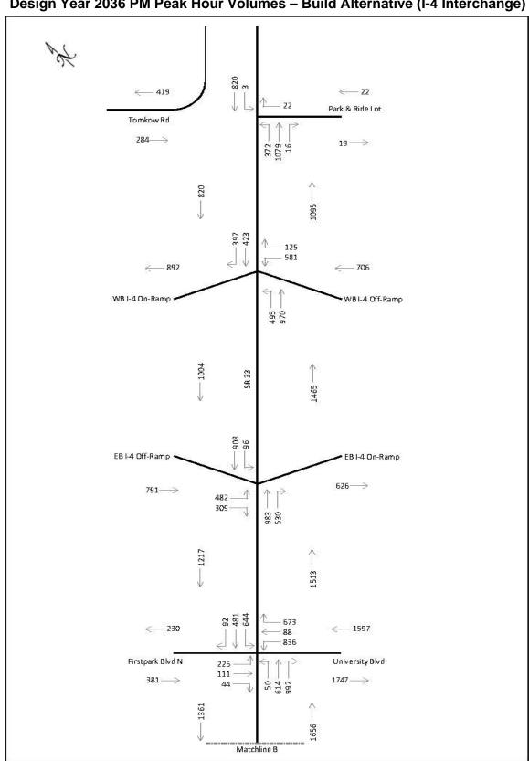
Figure 5-4 Design Year 2036 PM Peak Hour Volumes – Build Alternative (I-4 Interchange)
