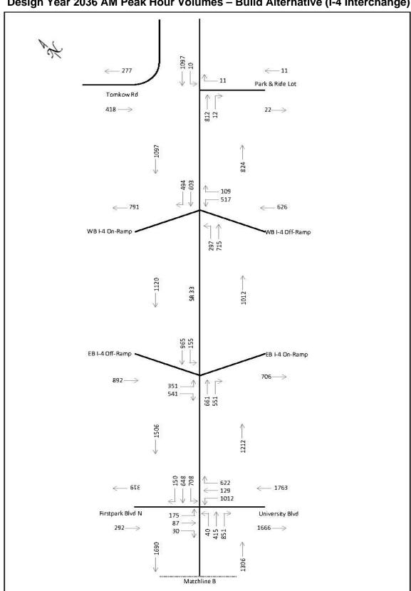
Figure 5-2 Design Year 2036 AM Peak Hour Volumes – Build Alternative (I-4 Interchange)
