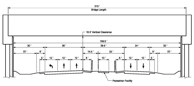
FIGURE 7-11: BUILD ALTERNATIVE NO. 2 PROPOSED TYPICAL SECTION – SR 33 UNDER I-4 LOOKING NORTH
