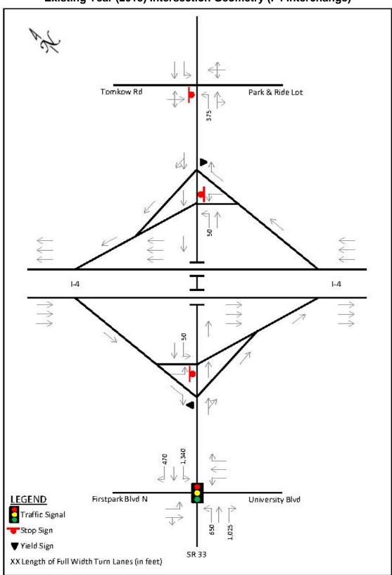
Figure 2-5 Existing Year (2013) Intersection Geometry (I-4 Interchange)
